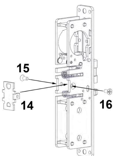
**NOTE:** The two springs need to rest on the protrusions on the inside of the cover plate.
