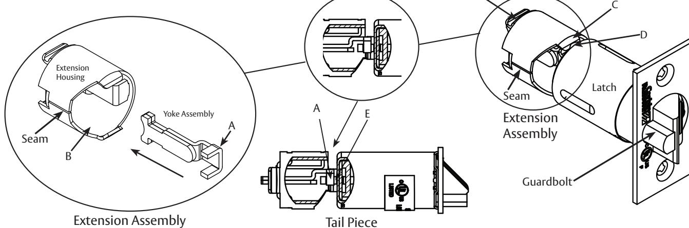
3. After assembly, the seam and cutaway "B" needs to be on the same side as deadlocking guardbolt. Then assemble sleeve to hold both latch and latch extension.
