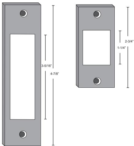
UL certified for up to 90 minute fire doors with clearance up to 5/16".
