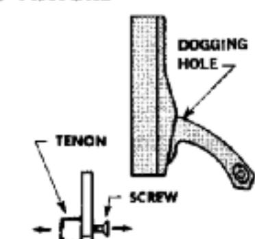
B. REMOVE TENONS FROM LEVERS — Using key furnished back out screw and remove tenon.
