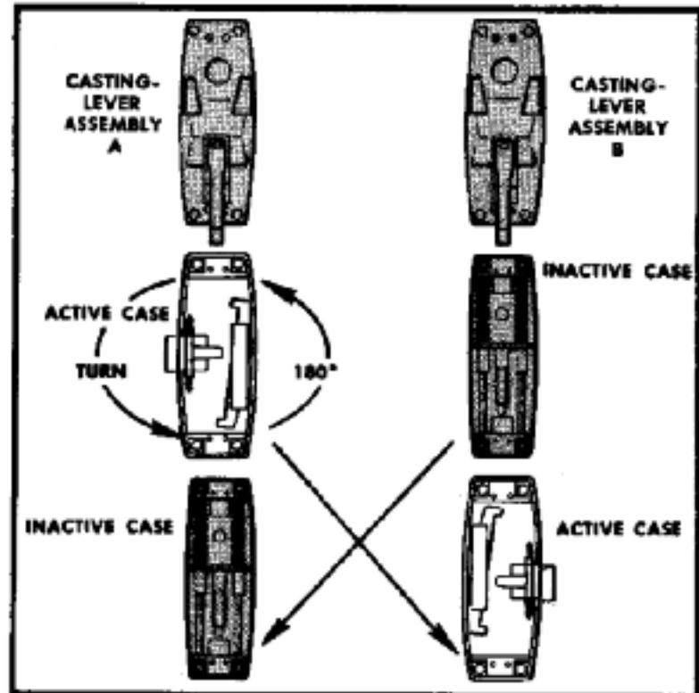
**D. REPLACE CASTING-LEVER ASSEMBLIES** — Put Casting "A" on *Inactive Case*, catching LEVER LIP under Post. Depress Bolt, push Slide-Bar (opposite latch UP, push bottom of Rocker away from latch, and position Casting "B" on *ACTIVE CASE* so **FINGER** is under Bolt Tail. SECURE WITH PHILLIPS HEAD SCREWS. DO NOT REPLACE CASE COVERS.
