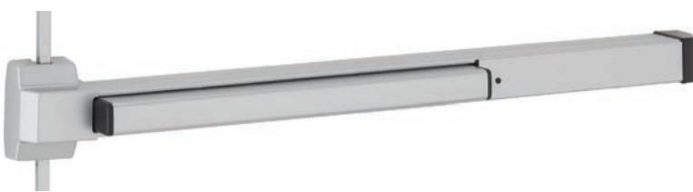
**2227 Surface mounted vertical rod exit device** for all types of single and double doors, UL listed for Panic Exit Hardware. Devices are ANSI A156.3 – 2008 Grade 1. Covers stock hollow metal doors with 86 or 161 cutouts. Fits door stiles as narrow as  $3\frac{5}{8}$ " (92 mm). The device is non-handed.
