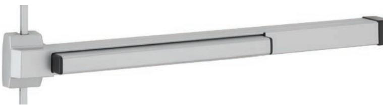
**2227-F Surface mounted vertical rod fire exit device** for pairs of doors up to 8' x 10' (2438 mm x 3048 mm), UL listed for Fire Exit Hardware. Devices are ANSI A156.3 – 2008 Grade 1. Fits door stiles as narrow as 3<sup>5/8</sup>" (92 mm). See opposite page for available outside trim and device functions. The device is non-handed.
