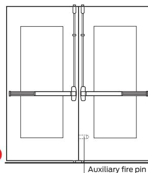
Two FEH vertical rods with auxiliary fire pin-LBR option (Don't use overlapping astragal on pair swinging same direction)
