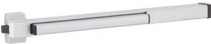
**22-F Rim fire exit devices** for all types of single doors up to 4' x 8' (1219 mm x 2438 mm) or 8' x 8' (2438 mm x 2438 mm) double doors with 9954 or 9854 mullion, UL listed for Fire Exit Hardware. Devices are ANSI A156.3 – 2008 Grade 1. Fits door stiles as narrow as 4<sup>3</sup>/<sub>8</sub>" (111 mm). The device is non-handed.
