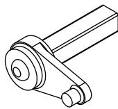
6. Indicator Spindle Cam - Coin
