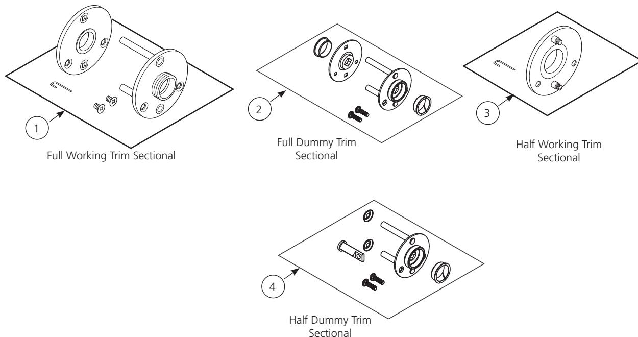
NOTE: Each adapter packet comes with appropriate size adapter plates & screws for door thickness as ordered.
