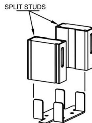
Before assembling Split Studs to header, snap nylon space pads onto top end of each stud. (Small pins fit into nailer slots and hold spacers in place). Nail studs into place as instructed in PK1200 assembly instructions.
