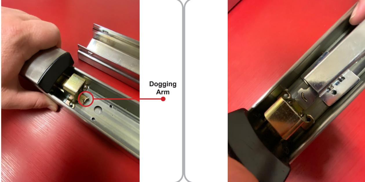
**4** Once in place pull back on the kit slightly to line up the mounting holes with the existing screw holes **Exit Device** and install (2) **Phillips mounting screws**.
