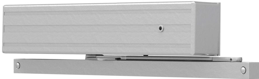
The 4310ME SENTRONIC® is a heavy duty, electrically controlled closer/holder designed to provide infinitely adjustable hold-open for fire and smoke barrier doors. Door is held open until current interruption releases mechanism and the door closes. Single lever (track) arm closer is specifically designed for interior doors. Choice of finishes, cylinder functions, and installation accessories meet virtually all life safety requirements. An ME provides only the closer / holder function.
