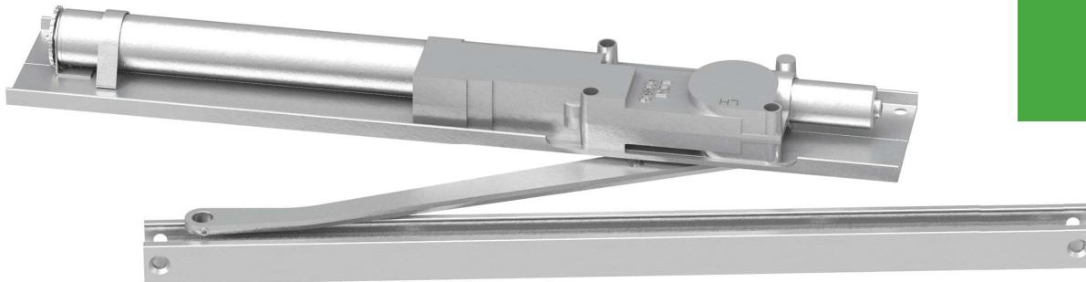
The concealed 2030 Series PACER® is a heavy duty closer designed to fit in a narrow, minimum 1-3/4" aluminum transom. The single lever arm and roller assembly provide smooth, quiet door control and the choice of finishes and track functions meet virtually all architectural requirements.
