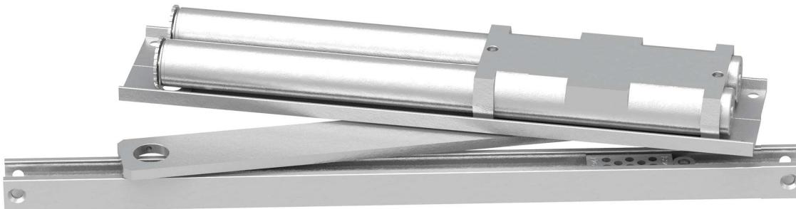
The concealed 6030 Series PACER® is a heavy duty, double acting closer designed to fit in a narrow, minimum 1-3/4" header. The single lever arm and roller assembly provides smooth, quiet door control and the choice of finishes and track functions meet virtually all architectural requirements. Installation at left illustrated with center pivot set (not included).
