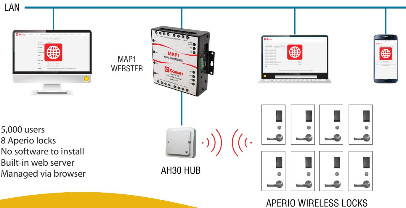
The MAP1 controller can be provisioned with Webster firmware to create an embedded web server supporting up to 8 Aperio wireless locks. Just plug it into the LAN network and use a standard browser on your PC or tablet to manage the Webster system. No software to install. Same price as a standard MAP1.
