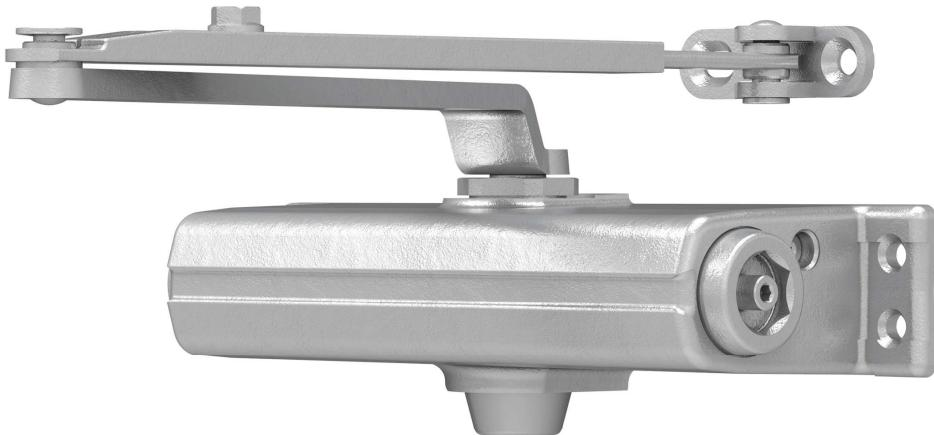
The 1260 is a light to medium duty cast iron closer designed to fit into the most common commercial foot print. The 1260 is adjustable for spring sizes 1-5. The 1260 also features a complete line of regular and extra duty arms, LCN's peel-n-stick installation templates, a convenient spring adjust pointer, and an optional Quick Fix™ bracket kit.
