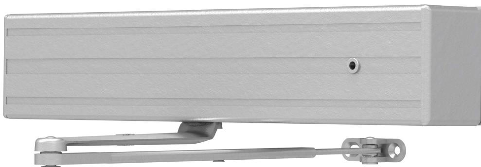
The 4410ME SENTRONIC® is a heavy duty, electrically controlled closer/holder designed to provide infinitely adjustable hold-open for fire and smoke barrier doors. Door is held open until current interruption releases mechanism and the door closes. Double lever arm closer is specifically designed for interior doors. Choice of finishes, cylinder functions, and installation accessories meet virtually all life safety requirements.
