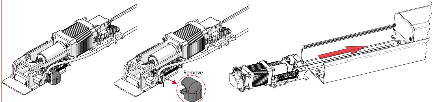
**5.** Tighten screws (4) securely, then test functions and adjust PTS location (see page 4). Once complete, install rear bracket, filler plate, and device end cap to finish the installation.
