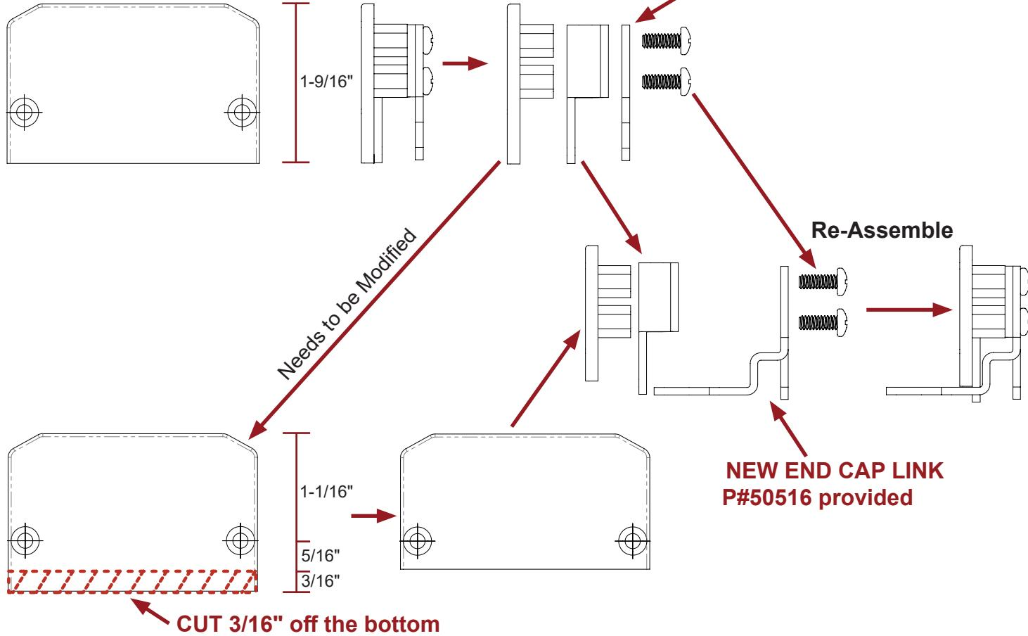
**3.** Re-install End Cap with New End Cap Link into the push pad housing.
