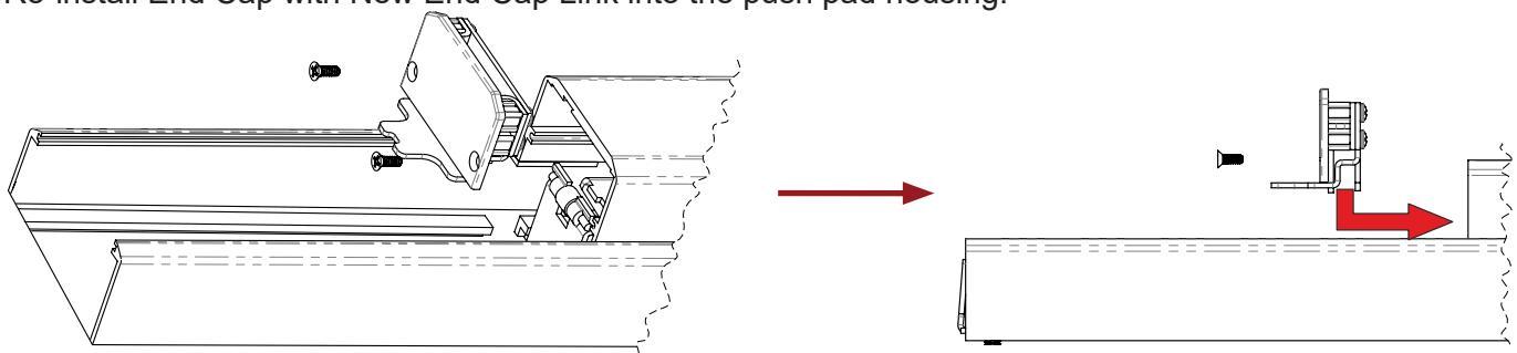
**4.** Remove the protection cap and discard, then slide motor assembly into the base rail channel
