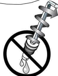
Do not remove valves from closer. Hydraulic oil will escape.
