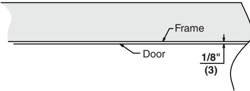
Templating is based on 1/8" gap between door and frame.
