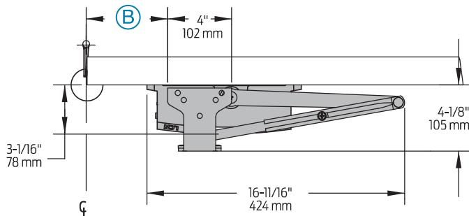
The 'A' dimension refers to the edge of the closer body to the center line of pivot or hinge.
