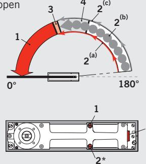
**NOTE:** Clockwise turns create a longer delay time with a slower closing speed. Turning valve completely clockwise creates hold open and eliminates delayed action.
